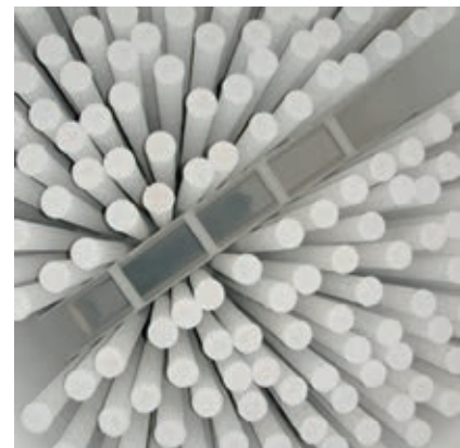
Hose filter, raw gas side
