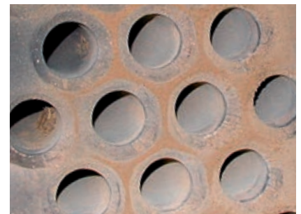
Gas tube boiler for waste heat recovery
